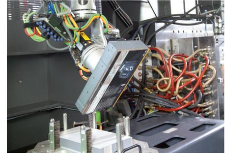
In-mould labelling (IML)
